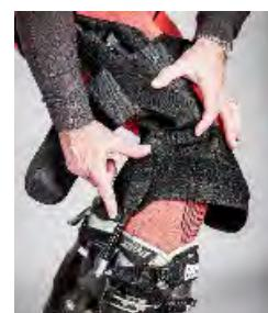
④ Slide the top of the telescopic rod into the hole in the bottom of the Harness connector. If you want to disconnect a leg from the harness, just press the brass button on the harness connector and pull-up the harness.
