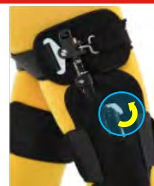
To switch off (dis-engage) the mojos, flip the switches up - then straighten your legs by sliding them backwards.
