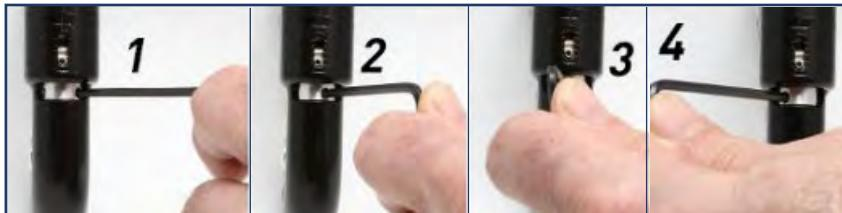
Insert the end of the Allen key in to the hole on the right and use the Allen key as a lever to rotate the Power Adjuster until the hole on the right has moved to the left. Repeat for each movement. Steps 1 to 4 above represent 1 movement.
